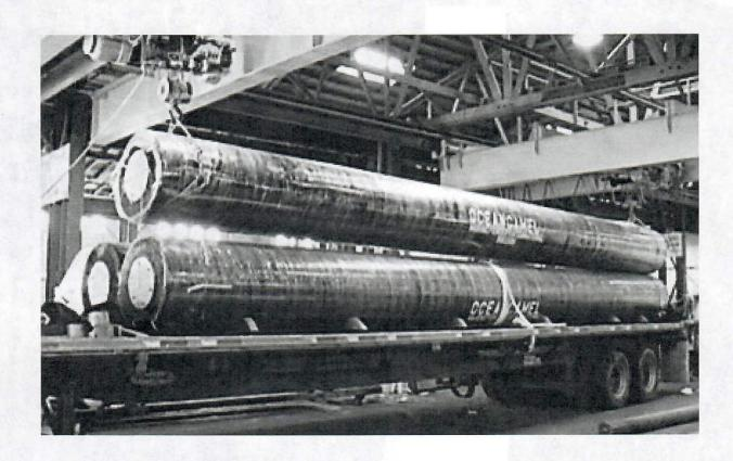
Ocean Camels<sup>™</sup> are composite floating camels designed to provide standoff between the vessel and the pier. Additionally, they are designed to distribute forces over a larger length of the pier structure to avoid point loads.
