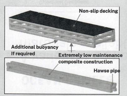
Ocean Camels™ are resilient composite camels are designed for a safe long life. Their outer abrasion resistant skin is constructed of the same proven materials as our Ocean Guard™ foam filled fenders. These non marking materials are also environmentally friendly.
